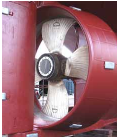
Before and after: New blades and nozzle gave a bollard pull increase from 19.1 to 23.6 metric tonnes
