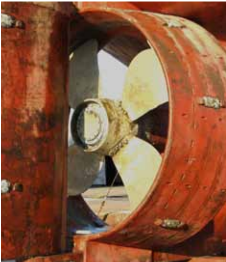
Before and after: New blades and nozzle gave a bollard pull increase from 19.1 to 23.6 metric tonnes
