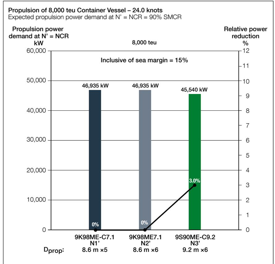
Fig. 10: Expected propulsion power demand at NCR for 24.0 knots
