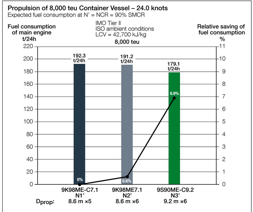
Fig. 12: Expected fuel consumption at NCR for 24.0 knots
