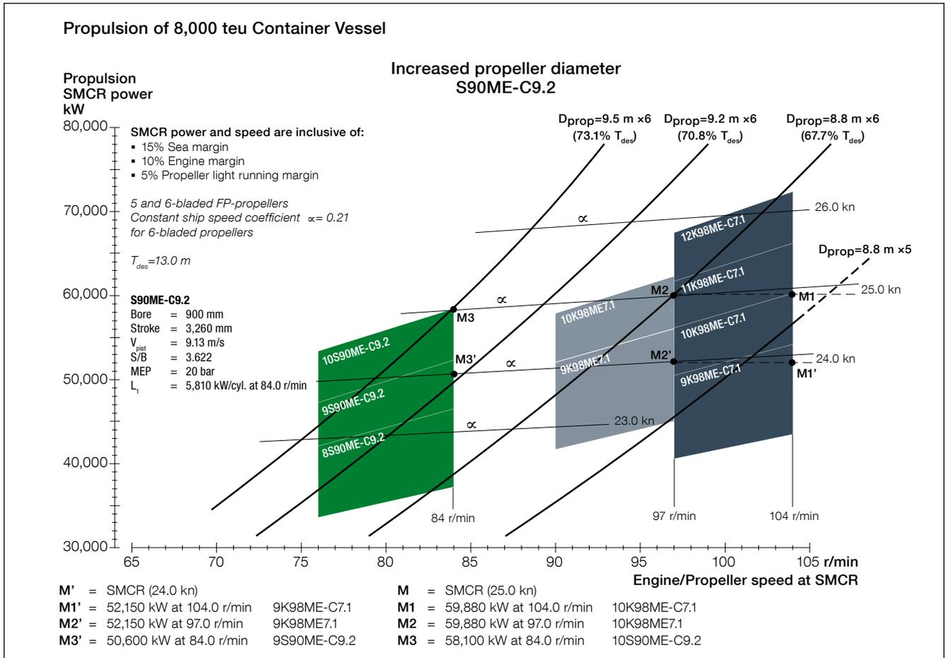
Fig. 3: Different main engine and propeller layouts and SMCR possibilities (M1, M2, M3 for 25.0 knots and M1', M2', M3', for 24.0 knots) for an 8,000 teu container vessel operating at 25.0 knots and 24.0 knots, respectively.
