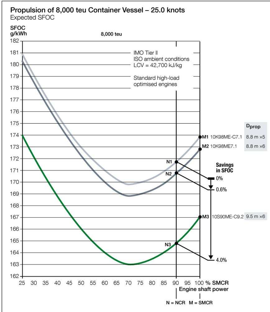
Fig. 5 shows the influence on the main engine efficiency, indicated by the Specific Fuel Oil Consumption, SFOC, for the three cases. N3 = 90% M3 for the 10S90ME-C9.2 has an SFOC of 164.8 g/kWh. The 164.8 g/kWh SFOC of the N3 for the 10S90ME-C9.2 is 4.0% lower compared with N1 for the derated 10K98ME-C7.1 with an SFOC of 171.7 g/kWh. This is because of the higher stroke/bore ratio of this S-engine type.
