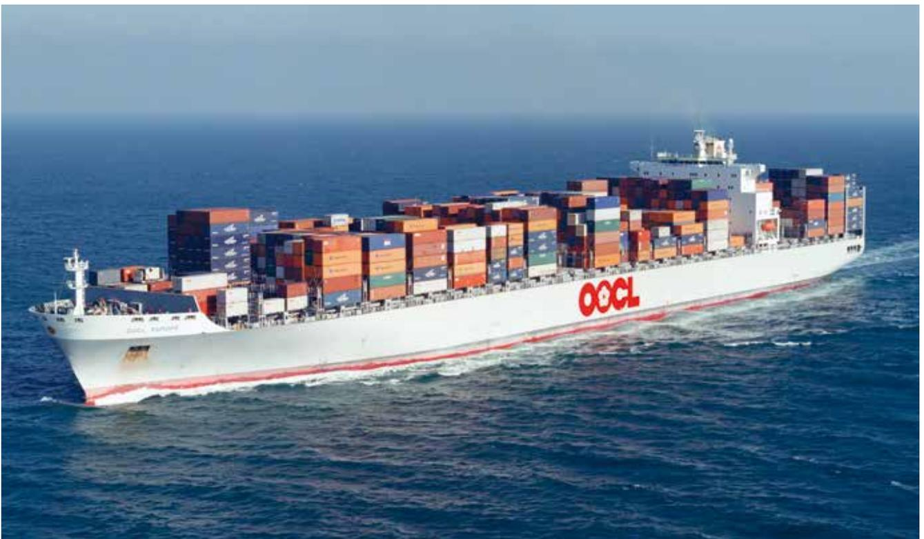
Fig. 1: An 8,000 teu container vessel
