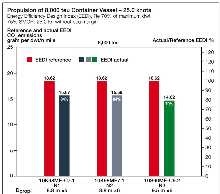
Fig. 7: Reference and actual Energy Efficiency Design Index (EEDI) for 25.0 knots
