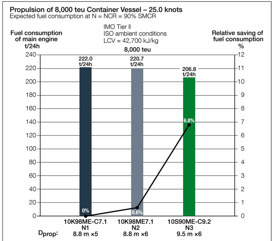
Fig. 6: Expected fuel consumption at NCR for 25.0 knots
