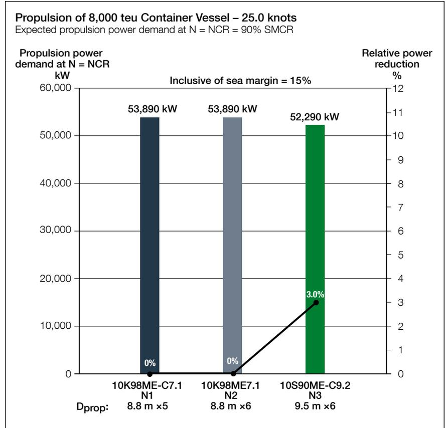
Fig. 4: Expected propulsion power demand at NCR for 25.0 knots
