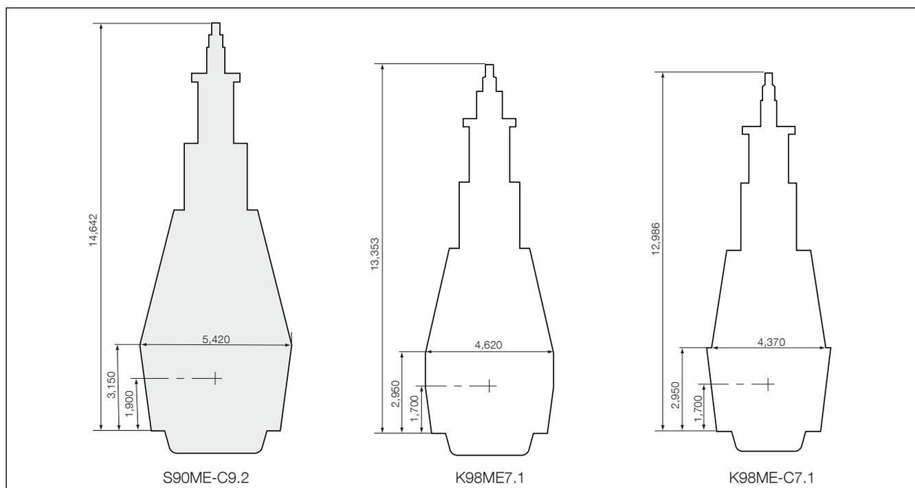
Fig. 2: Main dimensions for an S90ME-C9.2 engine and for other existing container ship engines
