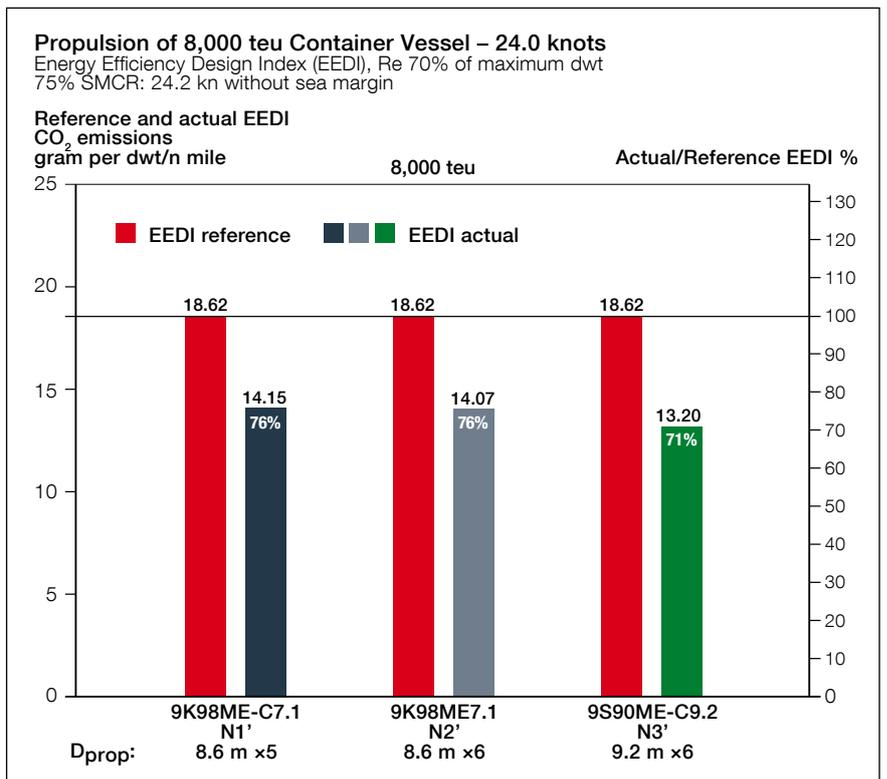
Fig. 13: Reference and actual Energy Efficiency Design Index (EEDI) for 24.0 knots
