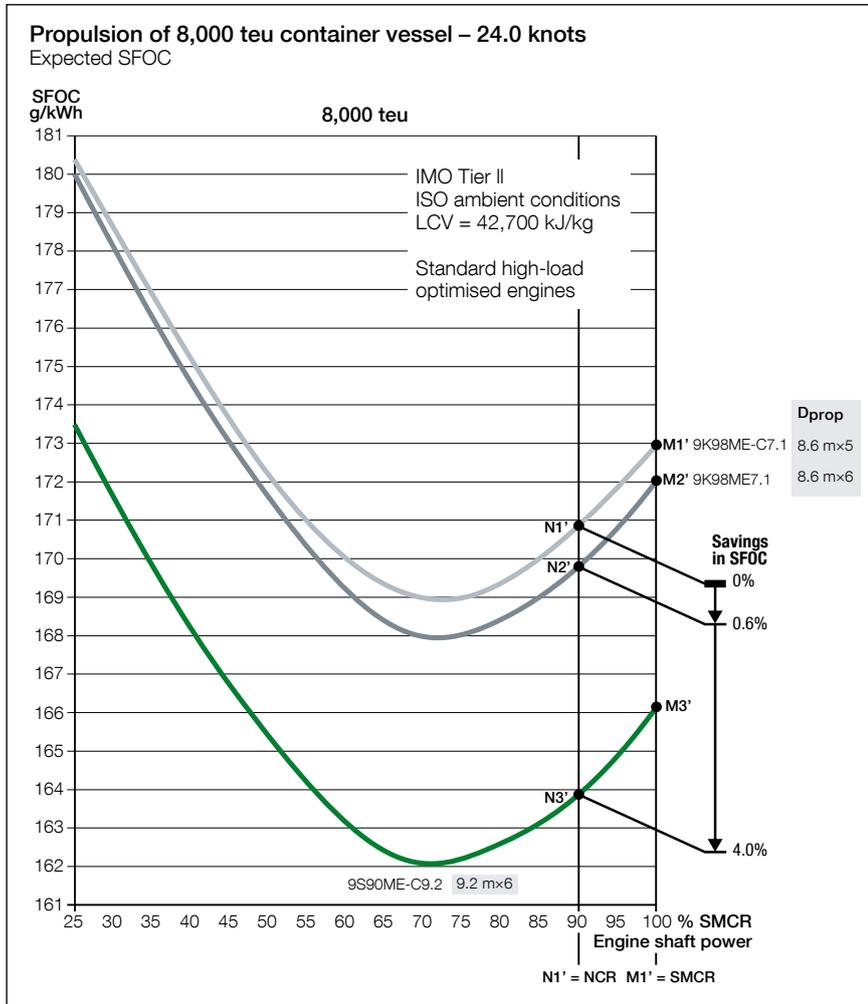
Fig. 11 shows the influence on the main engine efficiency, indicated by the Specific Fuel Oil Consumption, SFOC, for the three cases.  $N3' = 90\%$   $M3'$  with the 9S90ME-C9.2 has a relatively low SFOC of 163.8 g/kWh compared with the 170.7 g/kWh for  $N1' = 90\%$   $M1'$  for the 9K98ME-C7.1, i.e. an SFOC reduction of about 4.0%, mainly caused by the higher stroke/bore ratio of the S90ME-C9.2 engine type.
